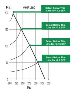
Note (Where fitted): Allow 30Pa for F7 Filter Allow 18Pa for M5 Filter
